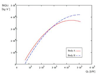
Fig. 2. Energy characteristics for body A and B of Pp-330/140-P55 steam boiler
